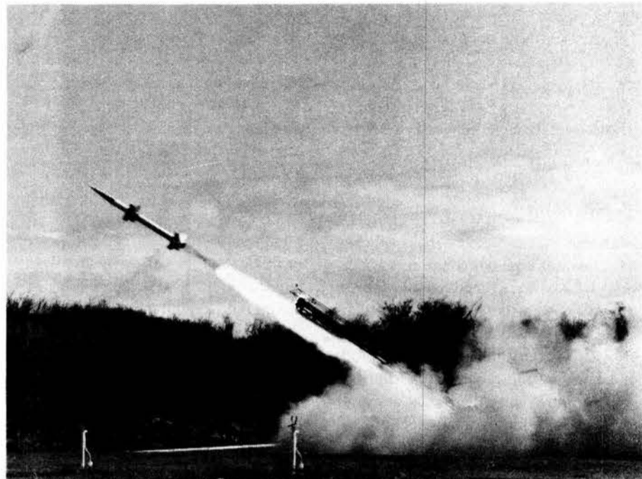
PENETRATOR DEVELOPED for high-speed water entry blasts off on a two-stage rocket at Barking Sands Facility (Kauai, Hawaii). Open-ocean impact conditions for the penetrator were a velocity of 1000 feet per second and an angle of 20°, relative to water surface.
